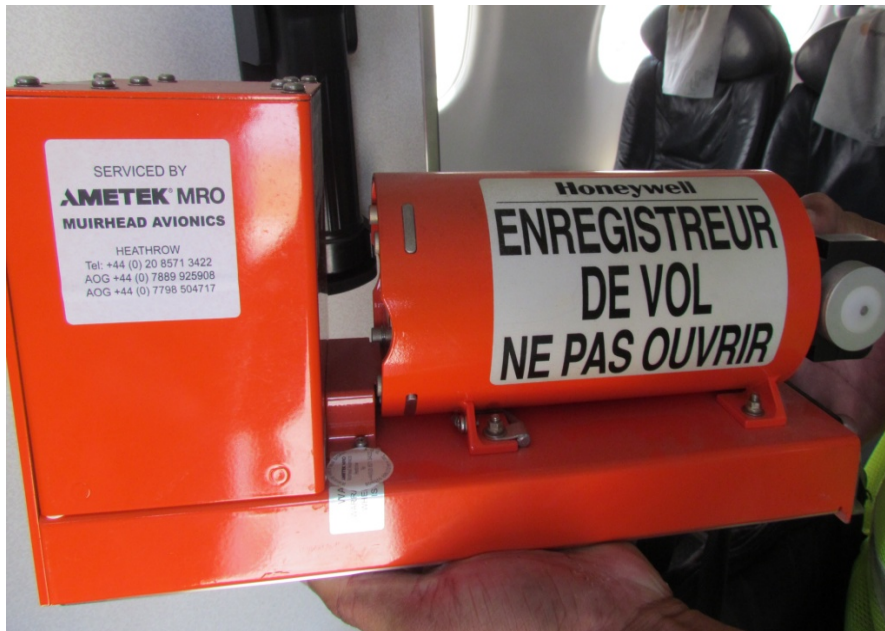
Figure (10) Digital Voice Data Recorder
