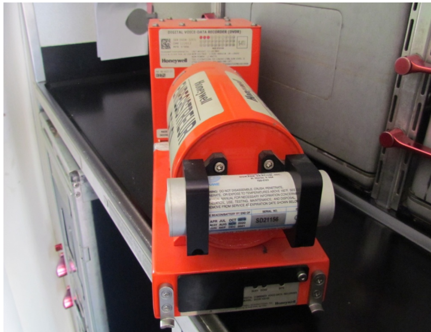
Figure (11) Digital Voice Data Recorder
