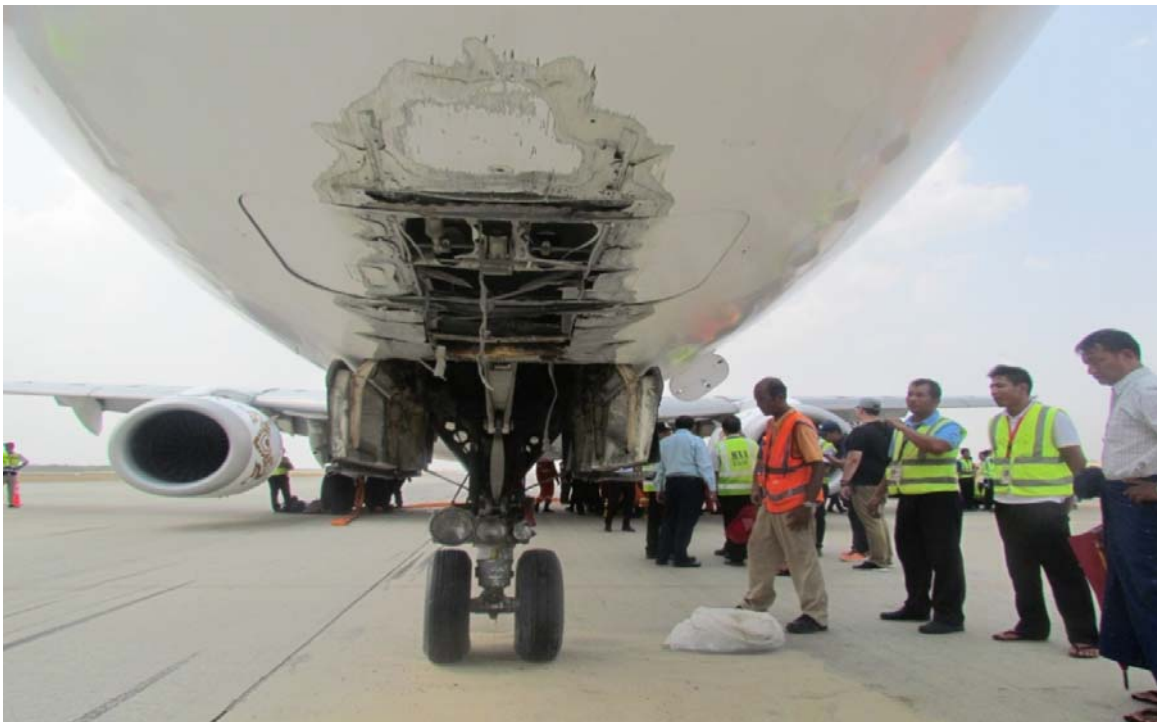
Figure (7) Damage to the aircraft Nose Landing gear section
