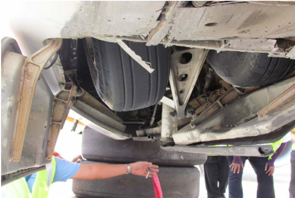
Figure (5) Closer view of the nose landing gear in the wheel well
