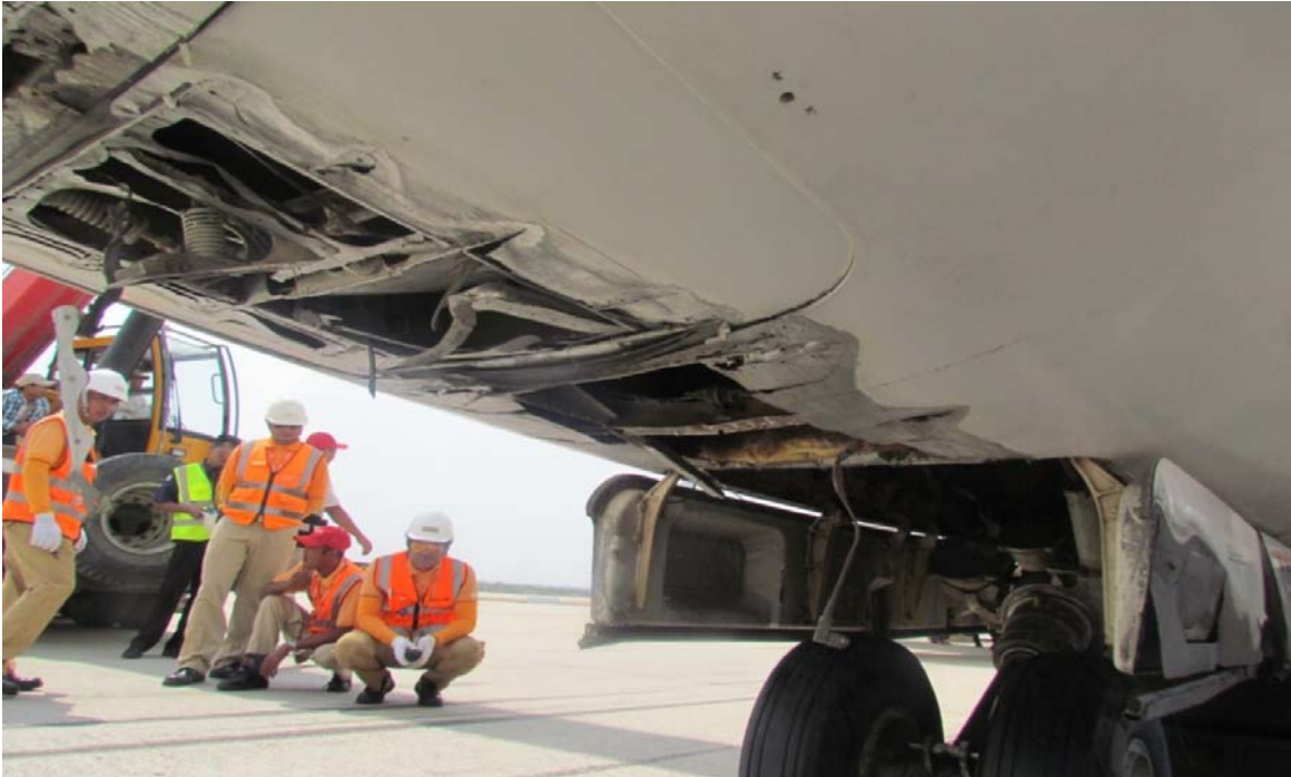
Figure (6) Damage to the aircraft Nose Landing gear section
