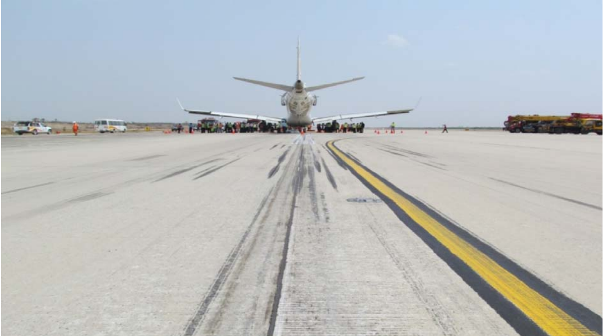
Figure (8) The Impact Marks on the runway
