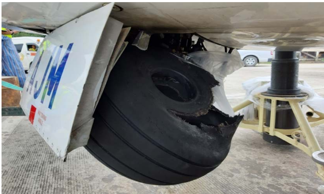
Figure (5) Both nose wheels thrown off from the axle with the no.(1) nose wheel tire hanging attached to the torque link
