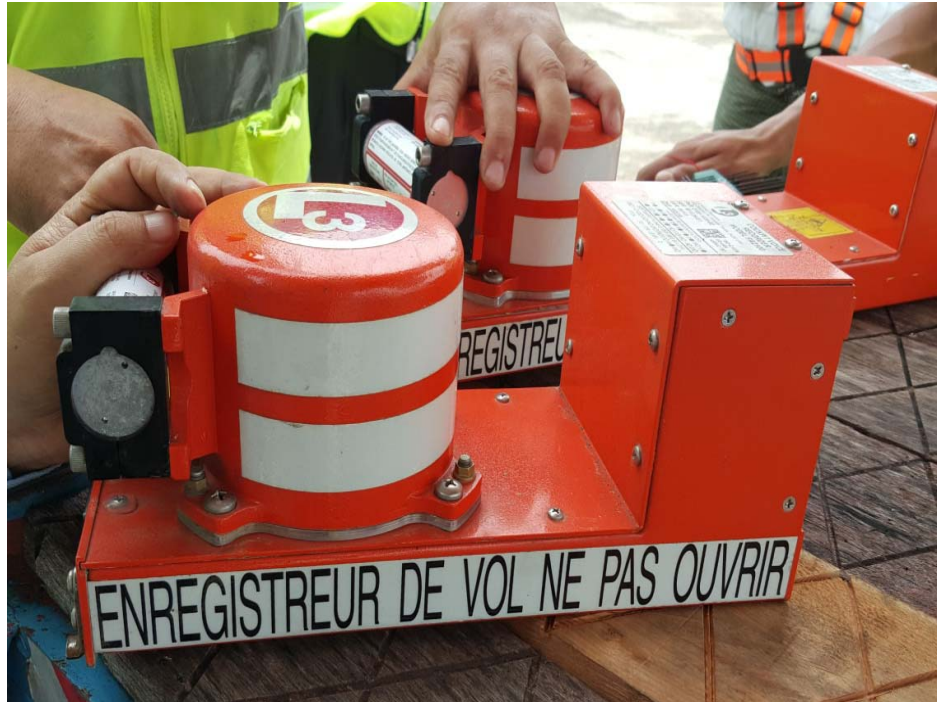
Figure (11) Cockpit Voice Recorder
