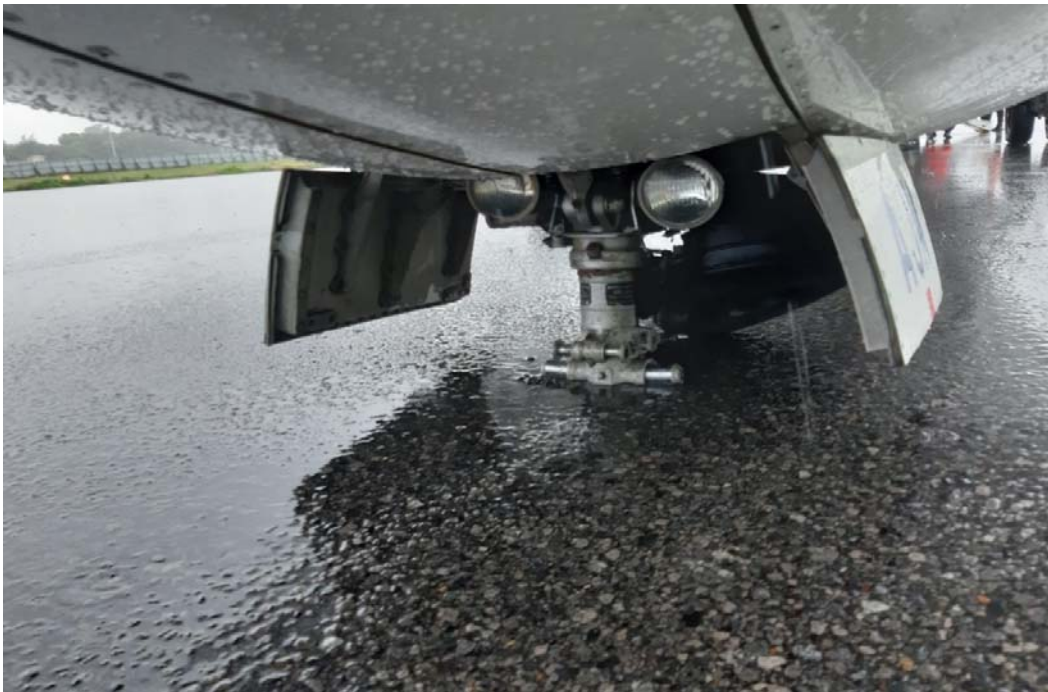
Figure (3) Nose landing gear damage
