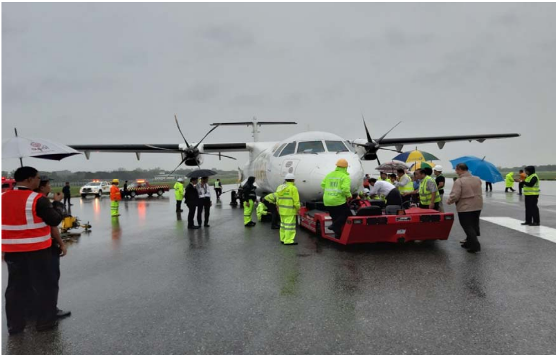
Figure (9) Disabled aircraft removal action
