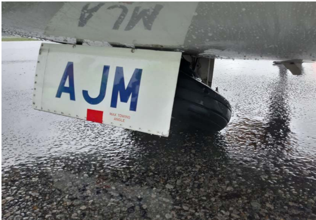
Figure (4) Both nose wheels thrown off from the axle with the no.(1) nose wheel tire hanging attached to the torque link
