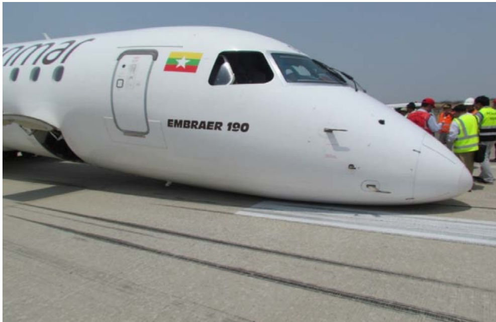
Figure (3) Closer view of the aircraft nose contact with the runway
