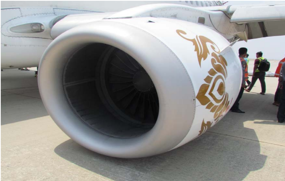
Figure (4) Left engine Cowling contact with the runway
