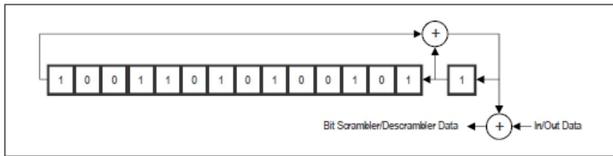
Figure D-6. Bit scrambler/descrambler
