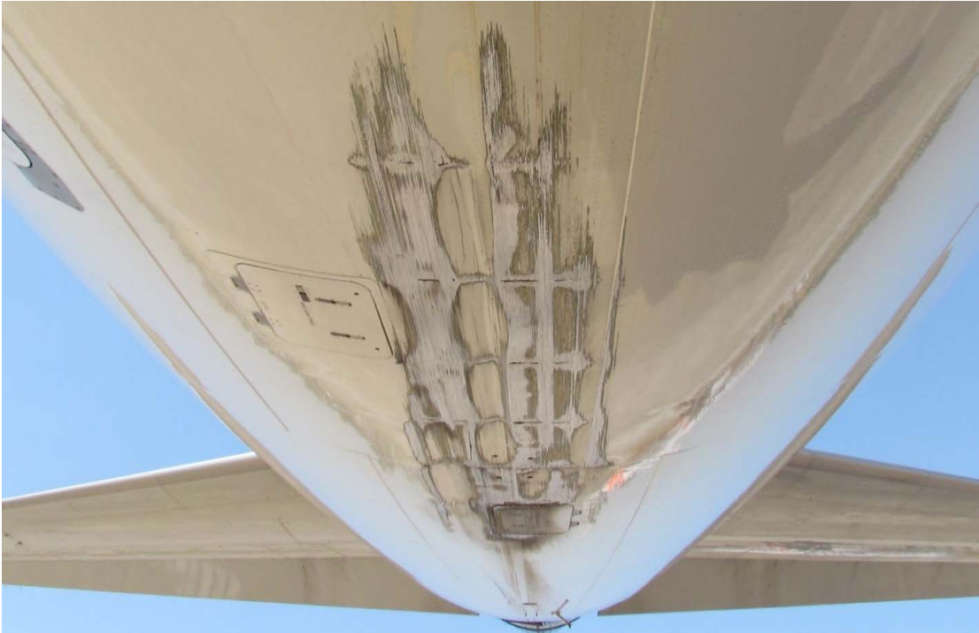
Figure (4) Scrape marks on aircraft tail section
