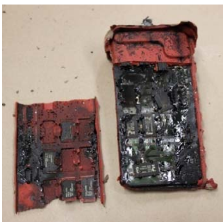
Figure 6: FDR memory module (accident module on left, normal module on right)
